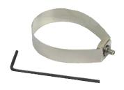
Clippard's stainless steel clamps are designed to be used with the Hall Effect and the reed switch. All clamps should be ordered based upon the size of the cylinder on which it will be mounted. The part numbers show the bore size using the numerical code. Each clamp is 0.375 wide stainless steel, and is equipped with a locking screw with #5-40 threads.
